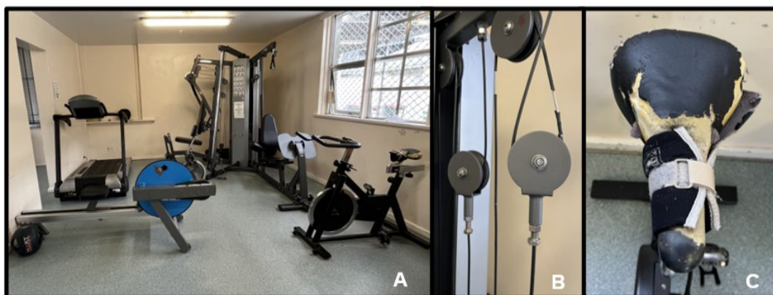
Figure 11. A) Exercise equipment in the Hartz gym area. B) Wear to cables of one on of the exercise machines in the women's prison. C) A close-up photo of the seat of the exercise bike in the Hartz unit.
